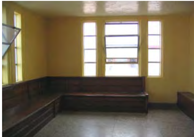
Figure 64: Zach's Bay comfort station lounge showing original cabinetry and terrazzo floor with replacement aluminum windows, 2004.
